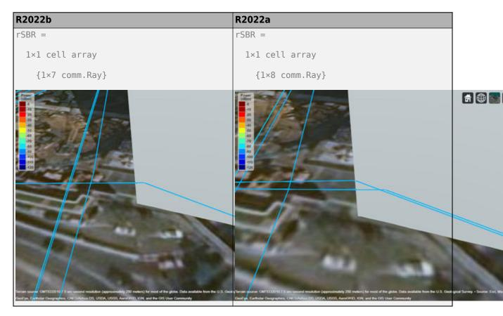
Paths calculated using the SBR method in R2022b more closely align with paths calculated using the image method. The image method finds all possible paths with exact geometric accuracy. For example, this code uses the image method to find propagation paths between the same transmitter and receiver.
